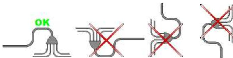
If a shaft is too long for the length required, it must be rolled up and never cut.
